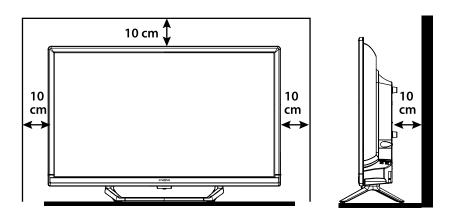
Install the display on a solid horizontal surface such as a table or desk. For ventilation, leave a space of at least 10 cm free all around the set. To prevent any fault and unsafe situations, please do not place any objects on top of the set. This apparatus can be used in tropical and/or moderate climates.
